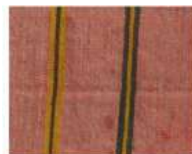
Fabric-1 Twill weave fabric woven on hand loom
