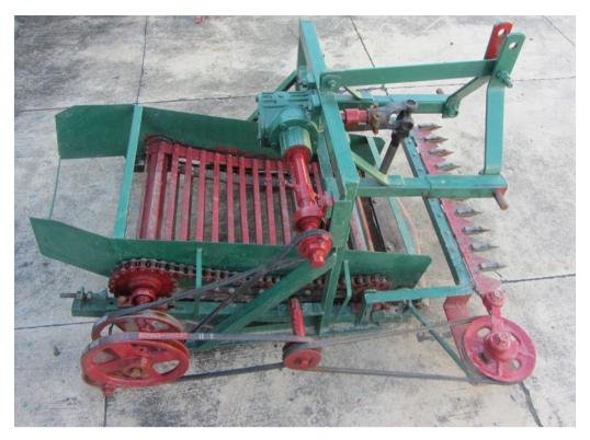
Plate 1. Developed onion digger with cutter bar topping unit
